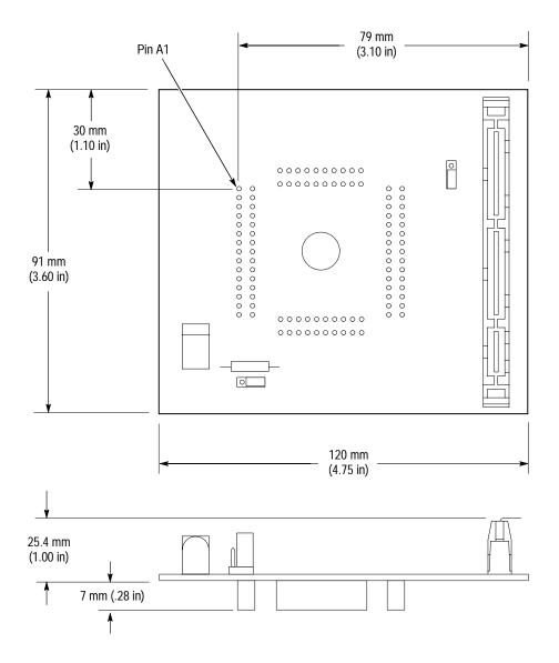
Figure 3–2 shows the dimensions of the 8XC196NP probe adapter. The figure also shows the minimum vertical clearance of the LAHDP2 probe cable.
