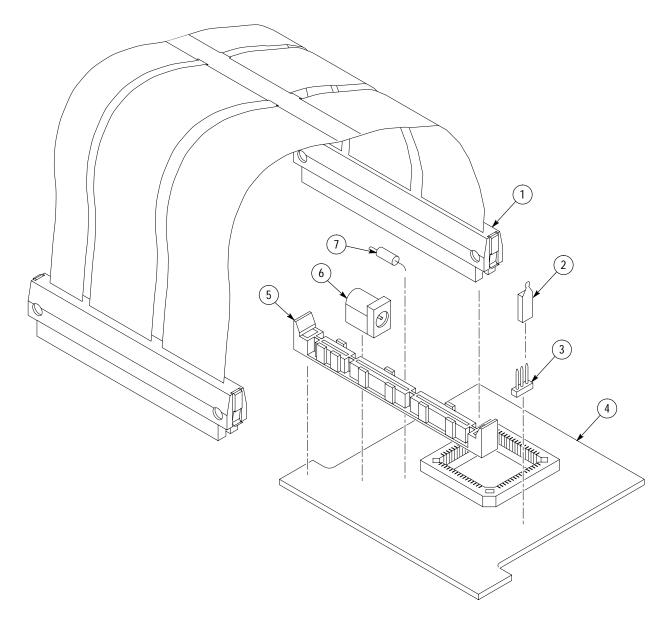
Figure 1: 8XC196NT probe adapter exploded view
