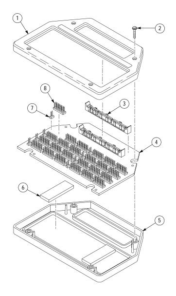
Figure 3: 192-Channel High-Density Probe exploded view
