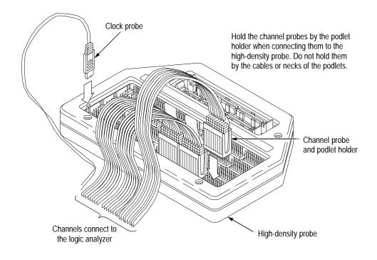
Figure 1–8: Connecting channel and clock probes to a high-density probe
