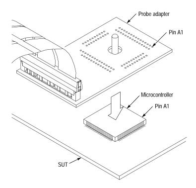
Figure 1-7: Placing a QFP probe adapter onto the microcontroller
