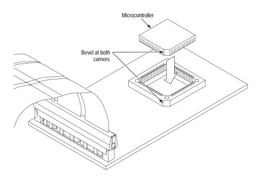
Figure 1-2: Placing a microcontroller into a PLCC probe adapter
