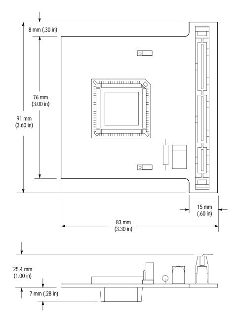
Figure 3–3 shows the dimensions of the 8XC196NT probe adapter. The figure also shows the minimum vertical clearance of the LAHDP2 probe cable.
