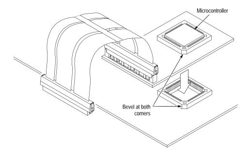
Figure 1–3: Placing a PLCC probe adapter onto the SUT
