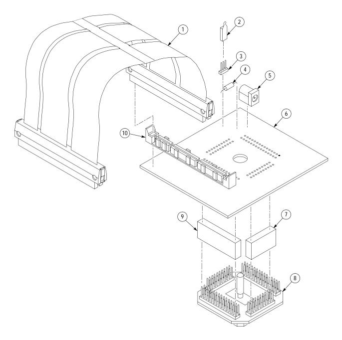
Figure 2: 8XC196NP probe adapter exploded view
